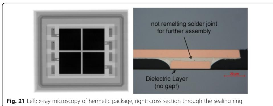
**Fig. 21** Left: x-ray microscopy of hermetic package, right: cross section through the sealing ring
