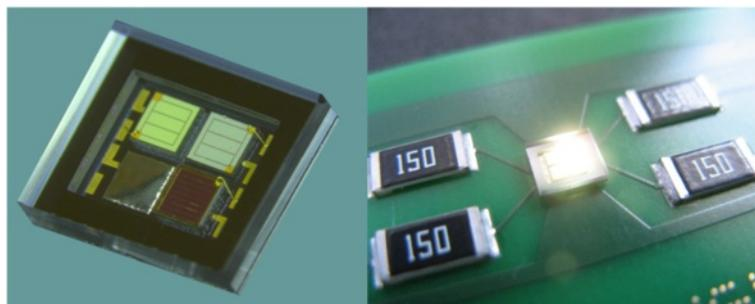
**Fig. 20** Left: hermetic RGB module, position of monitor diode is free, as not delivered in time, right: hermetic package on demonstrator board
