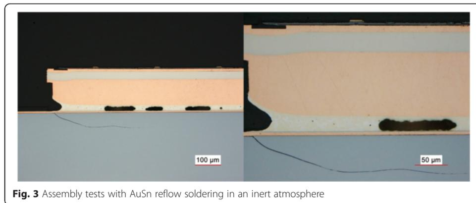
**Fig. 3** Assembly tests with AuSn reflow soldering in an inert atmosphere
