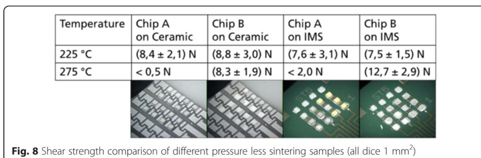
**Fig. 8** Shear strength comparison of different pressure less sintering samples (all dice 1 mm<sup>2</sup>)
