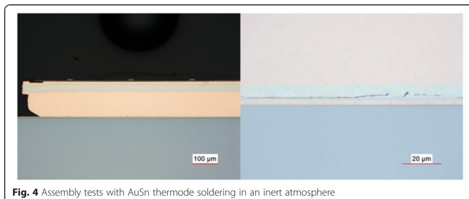
**Fig. 4** Assembly tests with AuSn thermode soldering in an inert atmosphere
