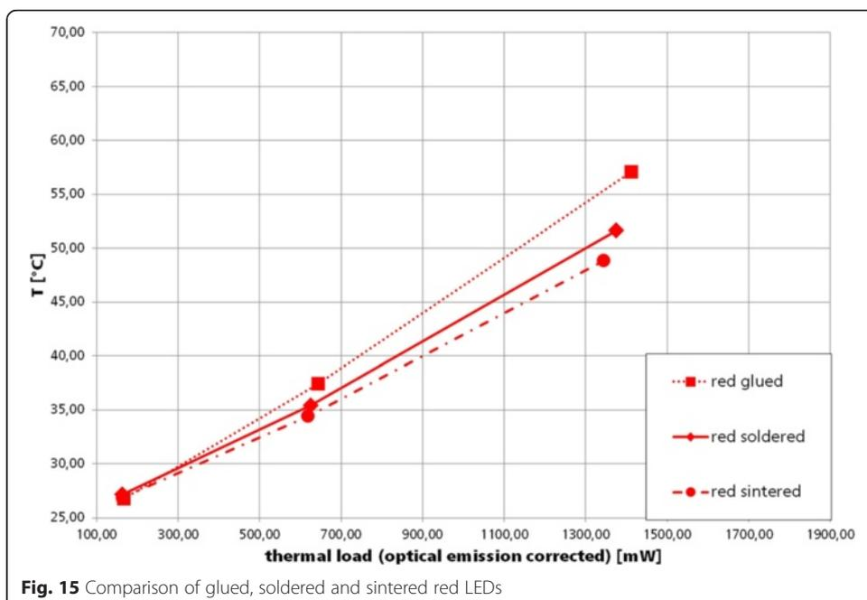
**Fig. 15** Comparison of glued, soldered and sintered red LEDs
