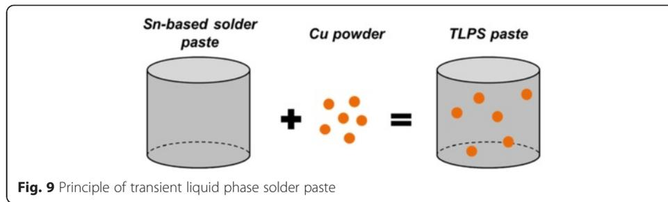
**Fig. 9** Principle of transient liquid phase solder paste
