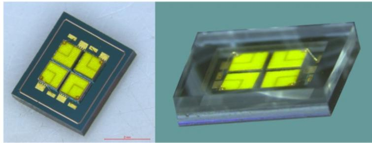
**Fig. 19** Left: exemplary substrate with four white LED and wire bonds, right: complete substrate with hermetic glass cap
