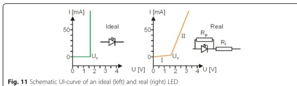
**Fig. 11** Schematic UI-curve of an ideal (left) and real (right) LED
