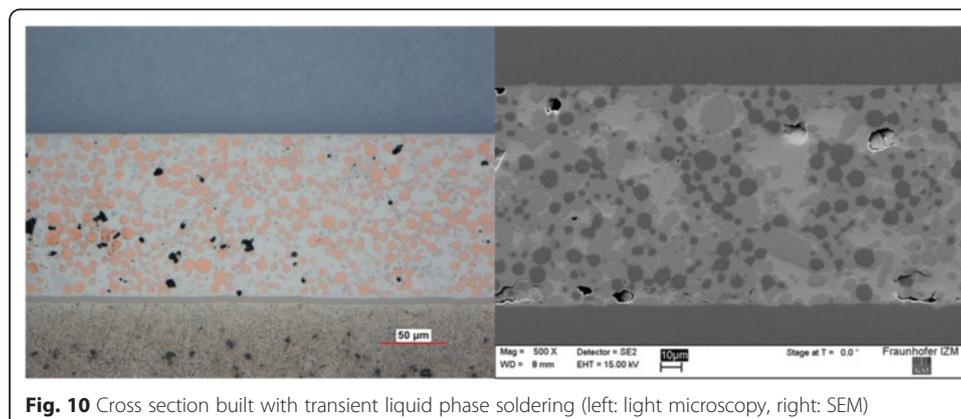
**Fig. 10** Cross section built with transient liquid phase soldering (left: light microscopy, right: SEM)
