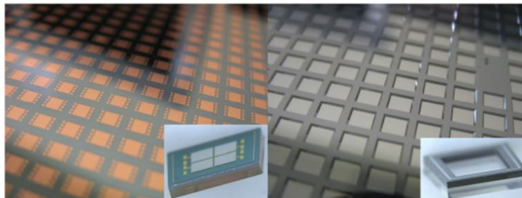
**Fig. 18** Left: substrate wafer, bottom view (insert: single substrate top view), right: glass cap wafer before metallization (insert: Single cap with metallization)
