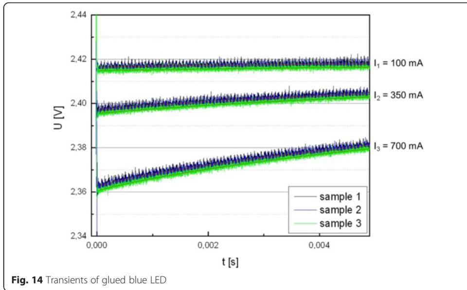
**Fig. 14** Transients of glued blue LED
