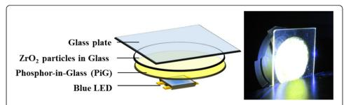
**Fig. 1** Configuration of a PiG specimen with a diffuser layer, and a photograph of white light generated from the specimen
