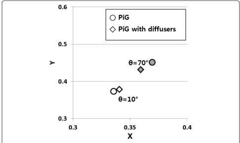
**Fig. 4** Color coordinates of white light from white LEDs using normal PiGs and PiGs with diffuser layers measured from the central part ( $\theta = 10^{\circ}$  from perpendicular direction) and at the periphery ( $\theta = 70^{\circ}$ )
