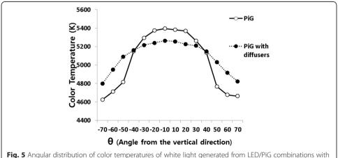
**Fig. 5** Angular distribution of color temperatures of white light generated from LED/PiG combinations with diffuser layers
