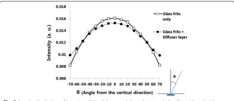
**Fig. 3** Angular distribution of intensity of blue light passed through sintered glass frits with and without  $ZrO_2$  diffuser layer. Neither specimen contained  $Ce^{3+}$ :YAG phosphors
