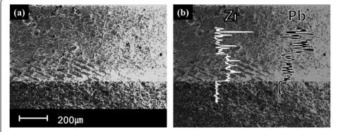
**Fig. 2 a** Secondary electron SEM image of cross section of PiG with a ZrO<sub>2</sub> diffuser layer. **b** Line profiles of Pb and Zr concentration analyzed by EDS
