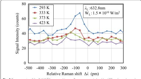
**Fig. 3** Raman spectra of the GaN-E<sub>2</sub><sup>H</sup> from one chip on a fluorescence-resin-less blue-LED package observed at various temperatures. Temperature of the blue-LED was kept constant and the LED was not operating (no emission light)
