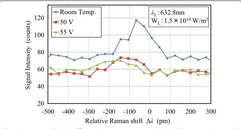
**Fig. 5** Raman spectra of the GaN-E<sub>2</sub><sup>H</sup> observed at various operating voltages. The LED operating voltages are of 50 V and 55 V. Raman spectrum from the same LED without operation at room temperature is also shown
