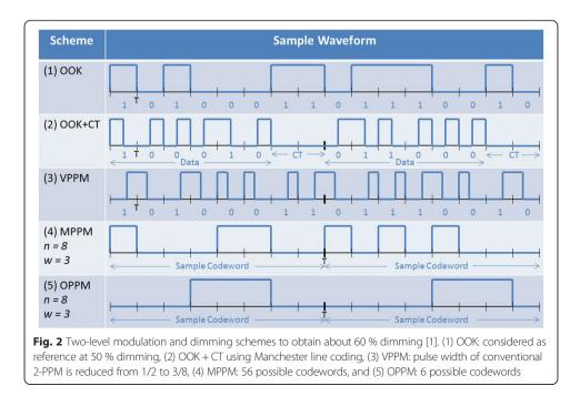
completely driven to its *on* state or *off* state, depending on whether one wishes to brighten above 50 % or dim below 50 %. The duration of the CT determines the precise proportion of peak power, *p*, that is emitted ( $p = P_{avg}/P_{pk}$ ).
