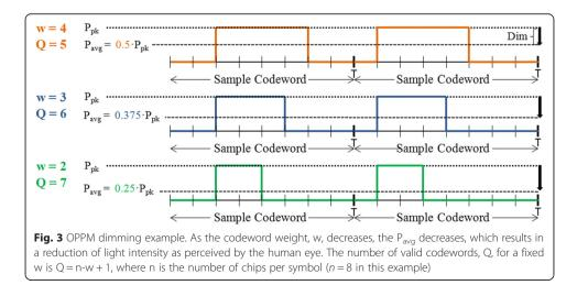
disadvantages with regard to light quality. Nonetheless, reference [5] demonstrates that OPPM with AM dimming fares well considering a flicker severity index as compared to OOK and VPPM. Future research is necessary to conclude if a hybrid of OPPM dimming using AM and the varying of codeword weights may inherit benefits of both techniques.
