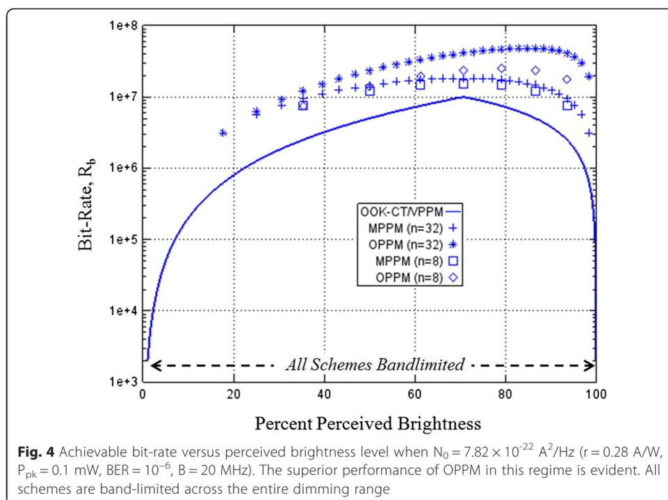
OOK-CT/VPPM. If brightness is increased to 98.4 % (31/32 of peak power), OPPM ( $n = 32$ ) drops to a bit rate of 19.4 Mbps, but still maintains superiority by achieving 16.3Mbps over MPPM ( $n = 32$ ) and 18.8Mbps over OOK-CT/VPPM. Dimming to 17.7 % (1/32 of peak power), MPPM matches OPPM at a bit-rate of 3.1 Mbps, which is 2.5Mbps greater than the bit-rate achieved by OOK + CT/VPPM. MPPM and OPPM are essentially both 32-PPM at this percentage (since  $w = 1$ ).
