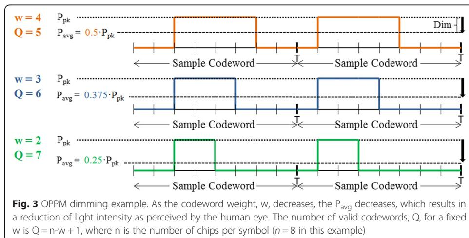
**Fig. 3** OPPM dimming example. As the codeword weight,  $w$ , decreases, the  $P_{avg}$  decreases, which results in a reduction of light intensity as perceived by the human eye. The number of valid codewords,  $Q$ , for a fixed  $w$  is  $Q = n - w + 1$ , where  $n$  is the number of chips per symbol ( $n = 8$  in this example)
