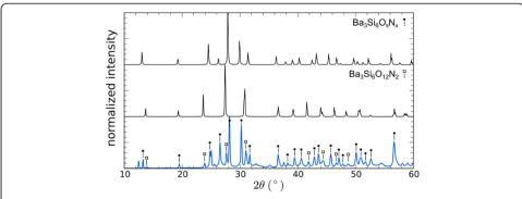
**Figure 2 XRD measurement of the top layer.** XRD measurement of the prepared green emitting top layer (bottom), compared with the calculated pattern for  $Ba_3Si_6O_{12}N_2$  (middle) and  $Ba_3Si_6O_9N_4$  (top) [27,28].
