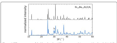
**Figure 1 XRD measurement of the blue phosphor.** XRD measurement of the prepared  $Sr_{0.25}Ba_{0.75}Si_2O_2N_2$ :  $Eu^{2+}$  powder (bottom), compared with the calculated pattern for  $Sr_{0.25}Ba_{0.75}Si_2O_2N_2$  (top) [19]. The black circles indicate reflections, possibly originating from  $BaSi_6N_8O$  [26].
