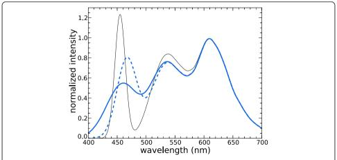
**Figure 9 Simulated LED spectra.** White LED spectra from simulations. Blue LED pumped (455 nm peak wavelength, thin solid line), UV pumped with a narrow band blue phosphor (467 nm peak wavelength, 40 nm FWHM, dotted line) and UV pumped with a broad band blue phosphor (460 nm peak wavelength, 65 nm FWHM, thick solid line).
