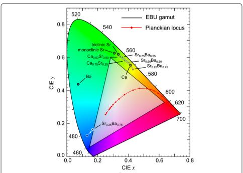
**Figure 4 Chromaticity diagram with MSi\_2O\_2N\_2:Eu^{2+} phosphors.** CIE 1931 chromaticity diagram with the color points of the  $MSi_2O_2N_2:Eu^{2+}$  family members. The white arrow indicates the color shift of the saturated blue  $Sr_{0.25}Ba_{0.75}Si_2O_2N_2:Eu^{2+}$  phosphor to the white due to the yellow emitting impurity phase. Color points of other phosphors from [7].
