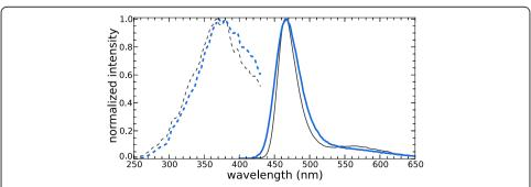
**Figure 3 Photoluminescence spectra.** Photoluminescence emission (excitation at 370 nm, solid lines) and excitation (emission at 466 nm, dashed lines) spectra of  $Sr_{0.25}Ba_{0.75}Si_2O_2N_2$ :Eu<sup>2+</sup>, measured at room temperature (blue, thick lines) and at 10 K (black, thin lines).
